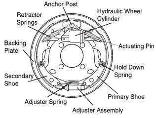
Figure 57. Hydraulic Brake Components
